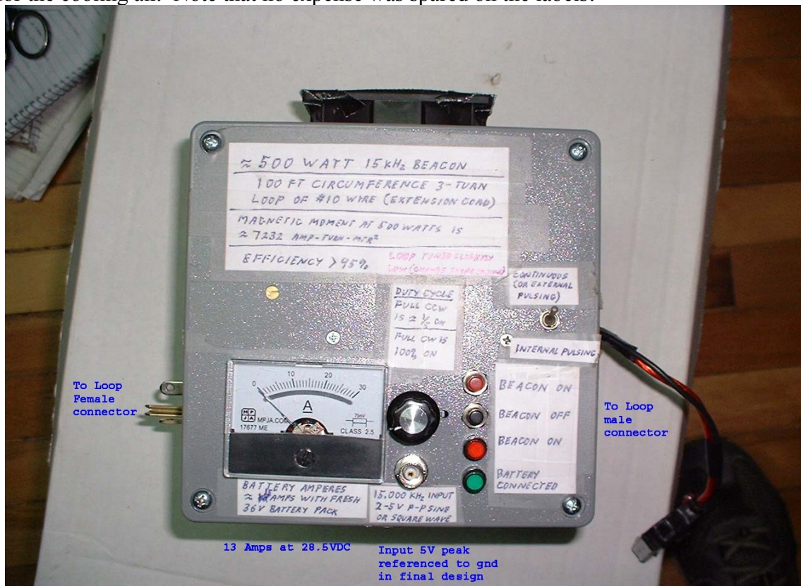
Figure 7 Prototype 500 Watt Beacon Amplifier
